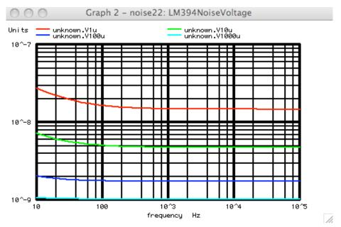
Spice likes to think in terms of power. Therefore a square root function needs to be applied to the output noise. In the output noise is onoise\_spectrum. The refered to input noise is the should equal the output noise divided by the gain.
