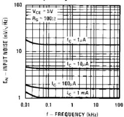
For the LM394, noise is pretty much set by the base resistance RB = 50 and the shot noise of a perfect transistor. At the 1mA current level the base current 1/f noise is just beginning to be felt. The match of the simulation and the Silicon may need some finer adjustments in the KF and AF values.
