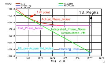
So given the model of the tuned circuit and the voltage across the tuned circuit, an integrated or accumulated line having a 20dB per decade slope can be drawn from where the clock frequency crosses the filtered and sampled pre-accumulated thermal noise level of the tuned circuit.
