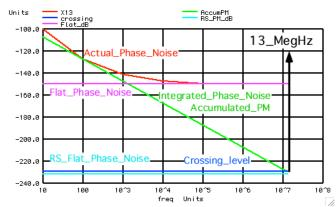
Now added a 20db/dec slope curve such that it is tangent to the Actual Phase Noise curve. That slope will be called the Integrated or Accumulated Phase Noise level. In an oscillator, the phase noise of each cycle gets accumulated over time. It crosses 13Mhz at -229 dB which will be called the crossing level.
