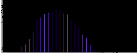
The ADC is 10Bit @100us. That is a 10KHz rate. But the data is being shipped serially at 115200 baud. Using 60Hz as a reference, looks like about 20 data points are being display over a 60Hz cycle. That is about a 1200Hz data rate. The overall Sample rate appears to be set by the serial data rate. That is 16.66msec/20 or 833usec per data point. If each data point is 5char "1024," @ 8 bits = 48000 bits/sec
