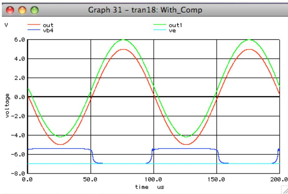
It had been common practice to stablize such an output stage by connecting a capacitor and small resistor to from the output to ground. The plot above shows the output with the stability compensation network in place.
