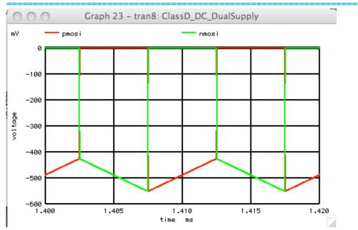
For the case of VCM = +2.5V and 50% duty cycle. Now VCM is supplying about 1.25W of power and RL is receiving it all.
