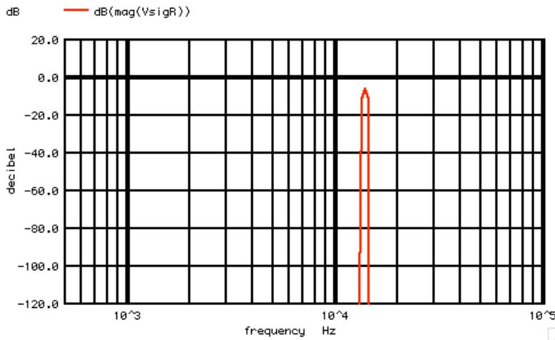
The wider spectrum can be narrowed a factor of two by just taking twice as long of a sample period. When this example used a 1msec sample period, the spectrum resolution is 1KHz, and the hanning windowed spectrum is spread out over three 1KHz frequency bins. When the sample period is 2msec, then the spectrum is spread out over 1.5KHz worth of frequency bins.
