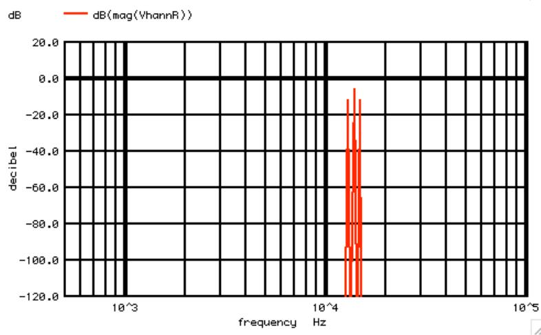
Now it is easy to see that there are clean signals at 13KHz, 14Khz, and 15Khz.
