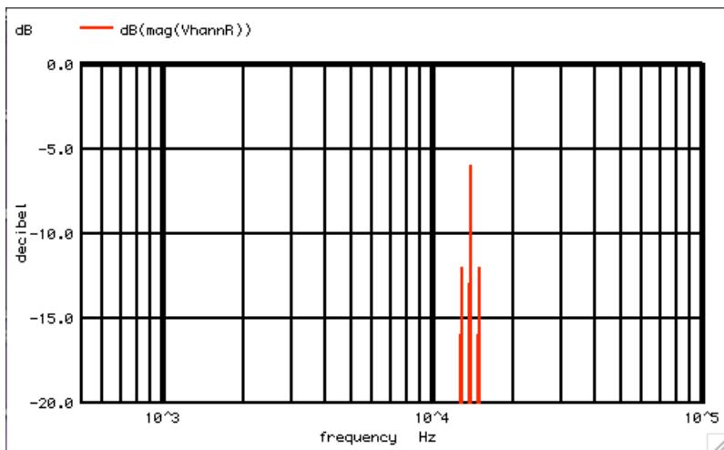
Now the 14kHz signal has been transformed to three frequencies. When thinking in terms of power, the two -6dB sidebands should increase the 14Khz power by about 22% or +1.76dB.
