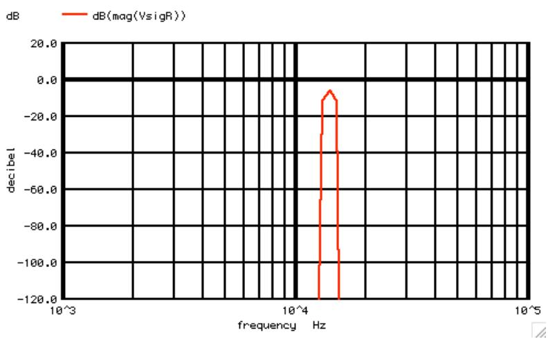
When looking at a hanning spectrum, every single frequency is going to be transformed into at least three frequencies. This should be taken into consideration when trying to extract a power value of such a spectrum. The side bands contribute about 22% to the total power.
