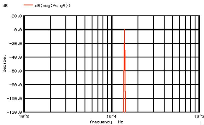
Since the input signal contains whole number of cycles in the 1msec sample period, the spectrum will have a clean signal at frequency bin number 14.
