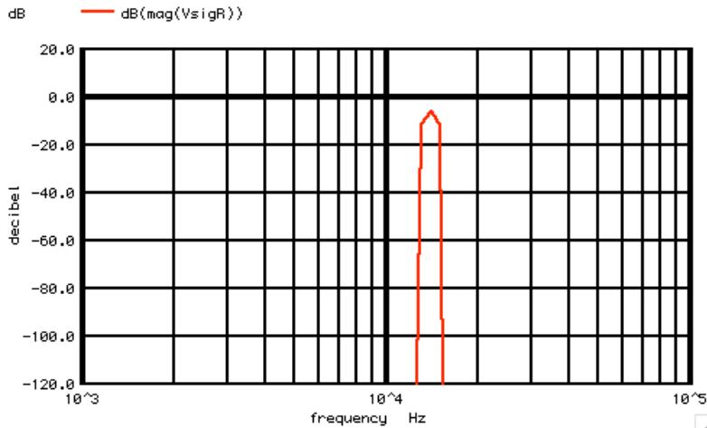
Lets sanity check the spectrum output by externally amplitude modulating the same signal with the Hann function, and redo the spectrum analysis again with a **rectangular** window.
