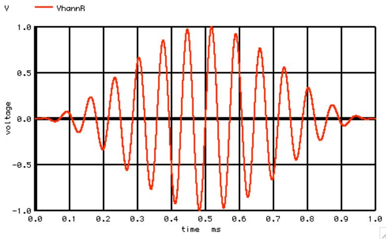
The input signal will look like so. The output of the spectrum comes out very close to the perfect 14KHz signal being processed with a **hanning** window.
