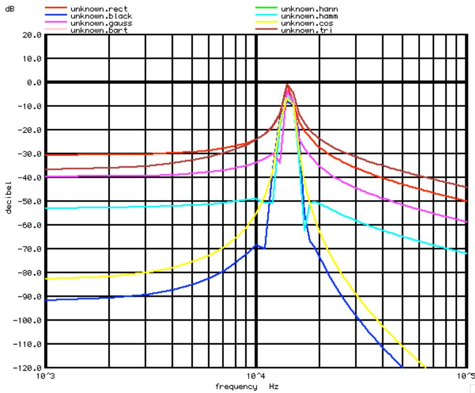
To plot several waveforms on the same plot, one has to call on the "unknown" plot. The **setplot new** statement creates this plot. In this case eight arrays/plots are assigned to it.
