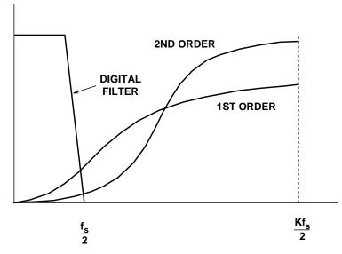
Figure 7: Sigma-Delta Modulators Shape Quantization Noise
