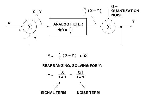
Figure 6: Simplified Frequency Domain Linearized Model of a Sigma-Delta Modulator
