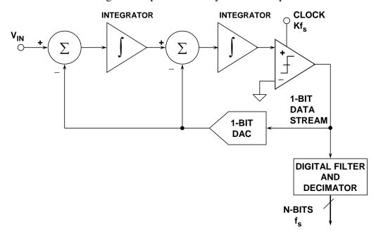
Figure 8: Second-Order Sigma-Delta ADC
