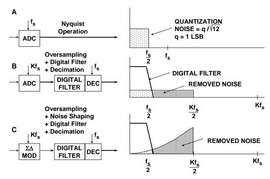
Figure 3: Oversampling, Digital Filtering, Noise Shaping, and Decimation
