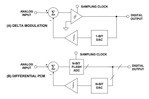
Figure 1: Delta Modulation and Differential PCM
