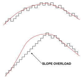
Figure 2: Quantization Using Delta Modulation
