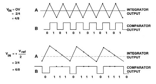
Figure 5: Sigma-Delta Modulator Waveforms
