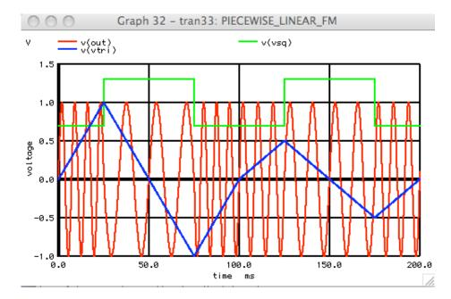
By Phase modulating with such a signal, it is obvious that the frequency modulation tracks the slope (or differential) of the input modulation signal. The PM signal has to FM the carrier first in order to PM the carrier.
