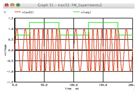
You will get a discontinuity in phase. But the FM can be done using Phase Modulation by first integrating the modulation signal.
