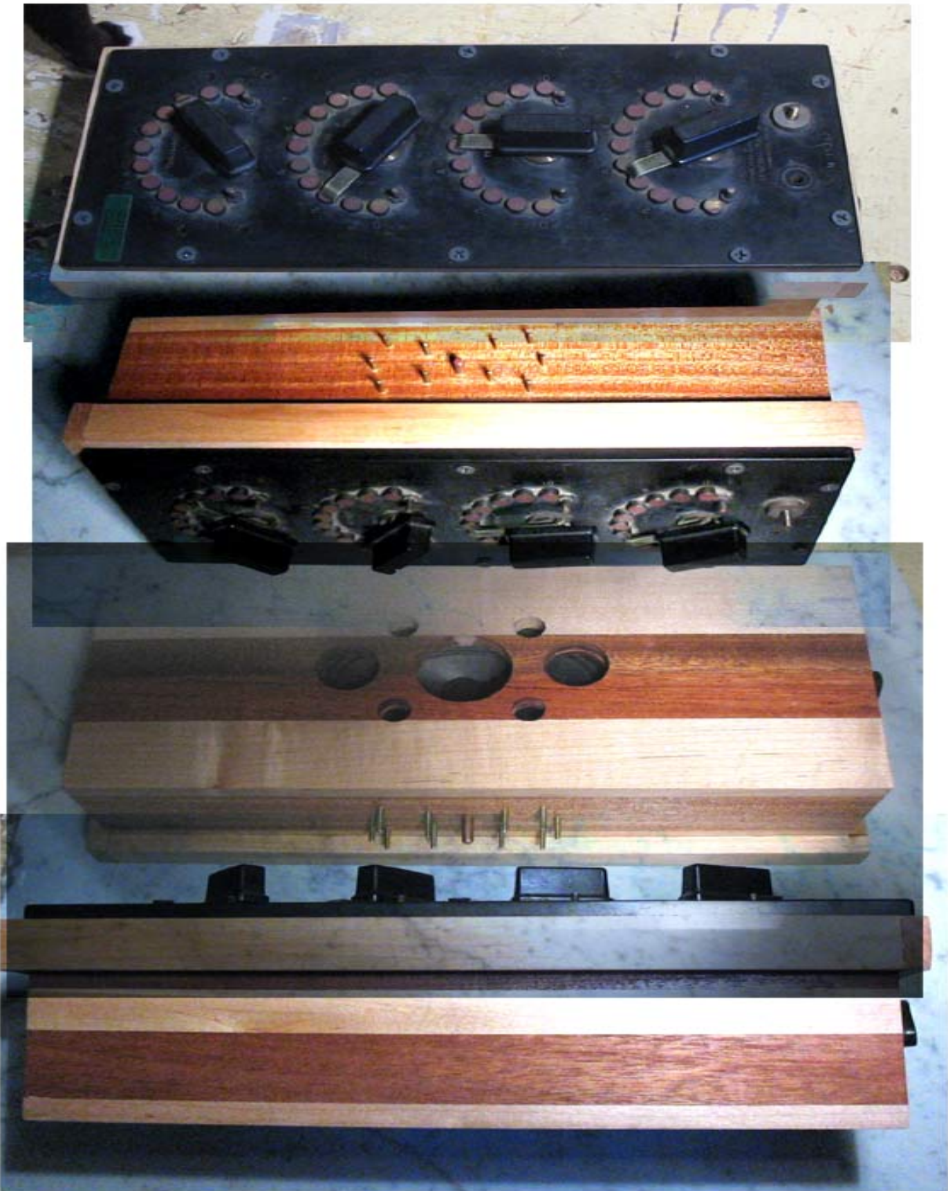
Here is a LIL SIDRASSI I put in a hardwood case with an antique dial system to switch hairy capacitors for multiple frequency system.
