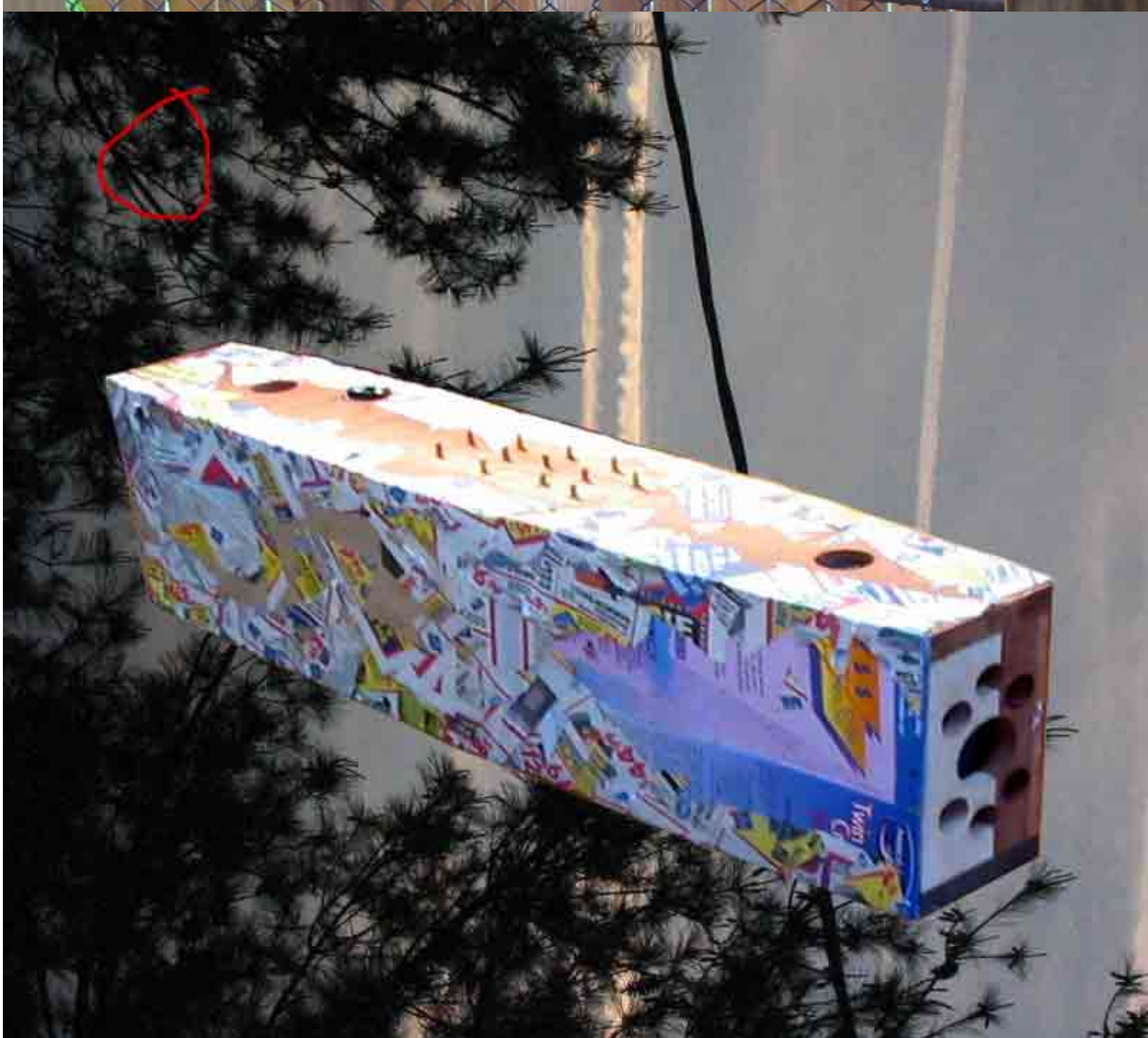
Here's my implementation of MR GRASSI. It has wooden boards for the top and bottom, then 2 drilled speaker planks, then cereal boxes for sides covered in papier mache
