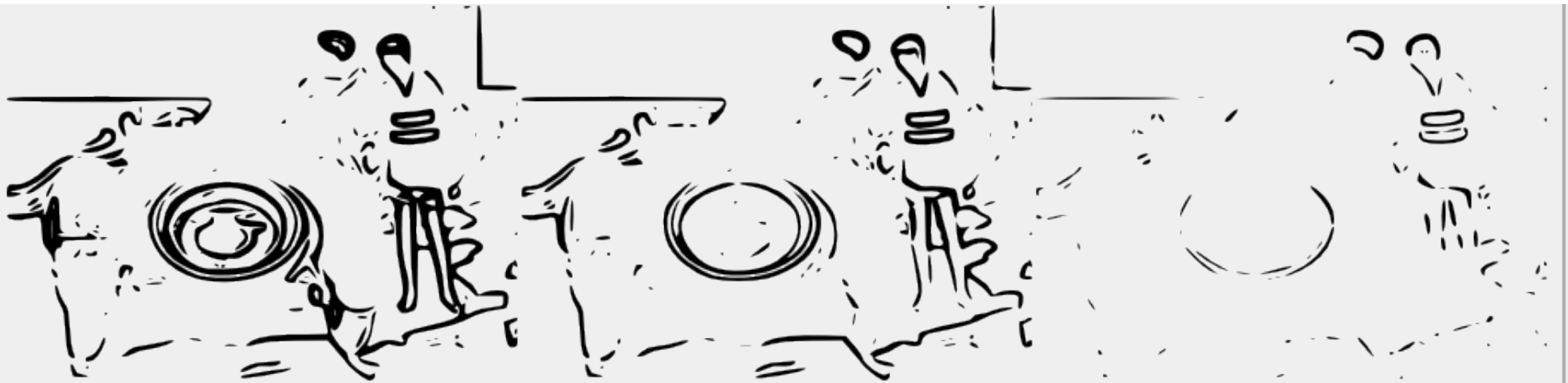
Edge detection for a color drawing. From left to right, the Threshold is 0.1, 0.5, and 0.9.
