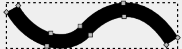
A filled path made from the stroked path by using the Stroke to Path command. It consists of ten nodes.
