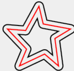
A star with both a linked inset and a linked outset. The original star (red) was modified after the creation of the linked paths.
