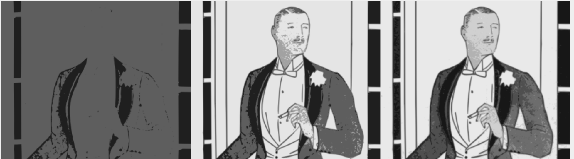
Multiple scans using the Colors option. From left to right, there are 2, 4, and 8 scans.
