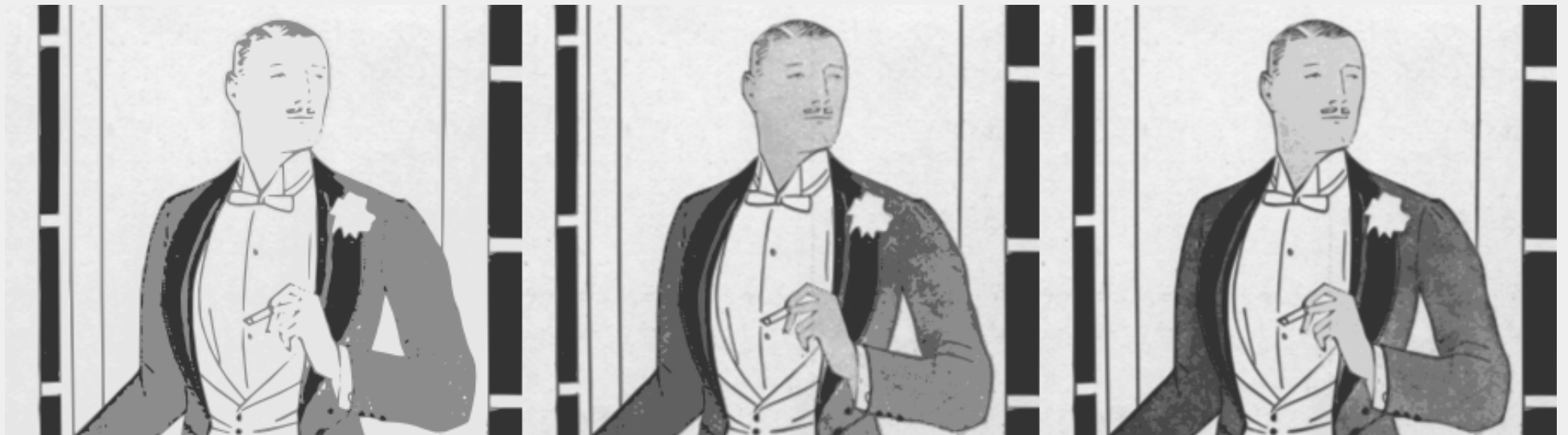
Multiple scans using the Brightness option. From left to right, there are 2, 4, and 8 scans.
