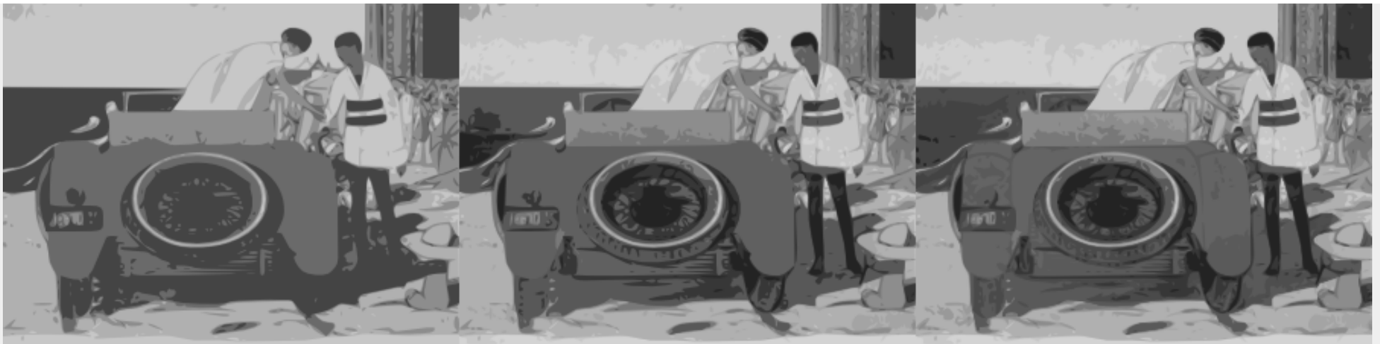
Multiple scans using the Grays option. From left to right, there are 5, 10, and 15 scans.
