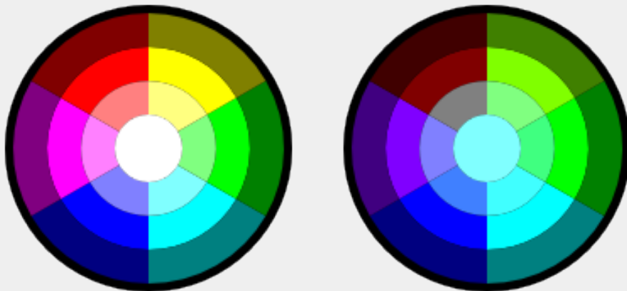
Left: Original colors. Right: Colors after applying the Color Custom effect with the specification that R should be divided by 2.
