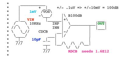
To take this 100dB of gain completely inside the chip, one needs to be able to do it using around 10pf capacitor. If it is possible to get something to act like a large enough resistor, then above 1kHz the RC attentuation will be greater than 100dB and the amplifier will be running open loop.
