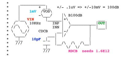
The circuitry used in the limiter circuit of a FM detector had long solved this problem using the circuit above. If the RC values could be made big enough, then the DC feedback could be one while at a high enough signal frequency the amplifier would be operating at open loop gain.
