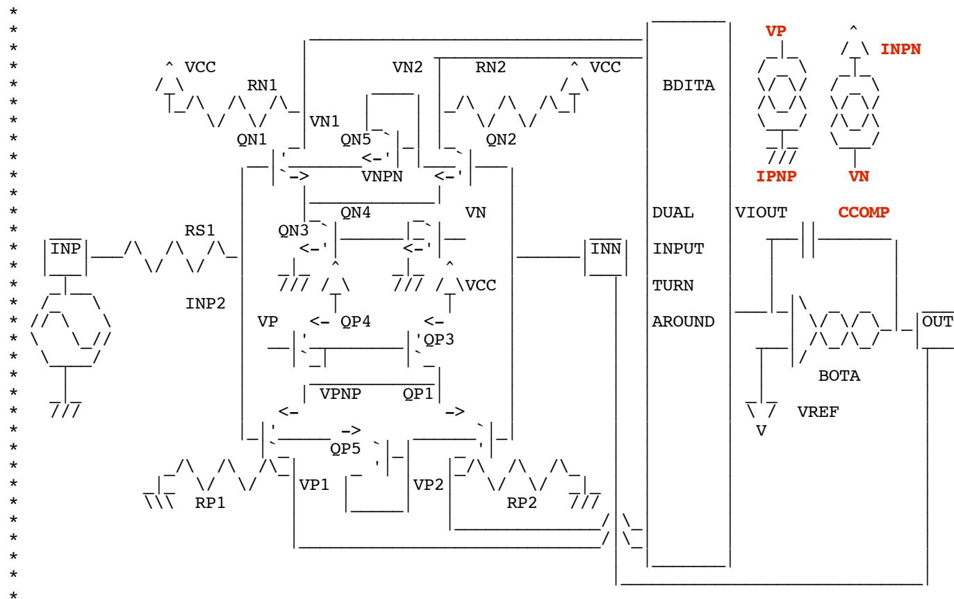
For the LM6142, the tail currents IPNP of the input stages was chosen by weighing an input bias current spec against a process beta spec. That chosen, the desired GainBandWidth for the Op Amp defines the magnitude of the compensation capacitor CCOMP used. This in turn
