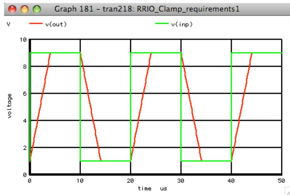
In the case of this simulation, current limiting resistor RS1 and clamp diodes QN5 and QP5 keep the voltages across the input transistors to within reason during the slewing period.
