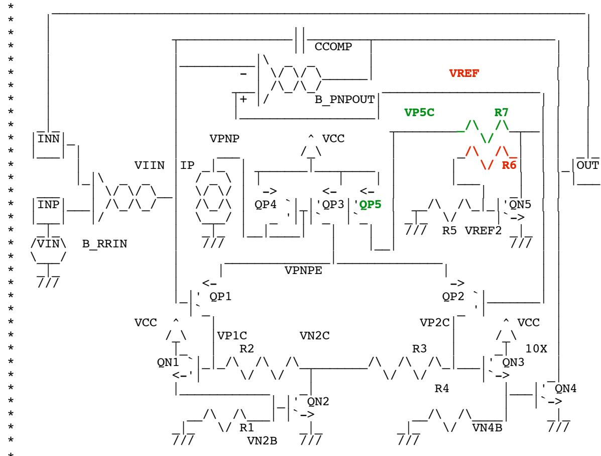
Above 5 volts a current source biases up a diode multiplier to provide a stable VREF. The plot of VP5C and Vref versus VCC shown below somewhat resembles the LM6142. Transistor QP5 is set up to saturate such that a 2.4V supply voltage generates a VREF which is at 1.2V.
