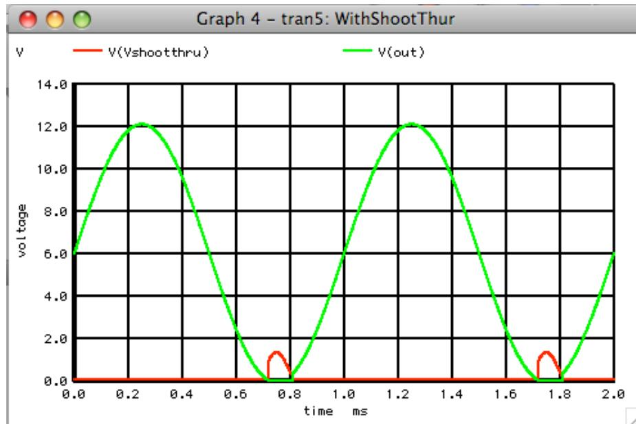
This means every time the output hits one of the rails, an supply current spike will happen which is referred to a a shoot thru current.
