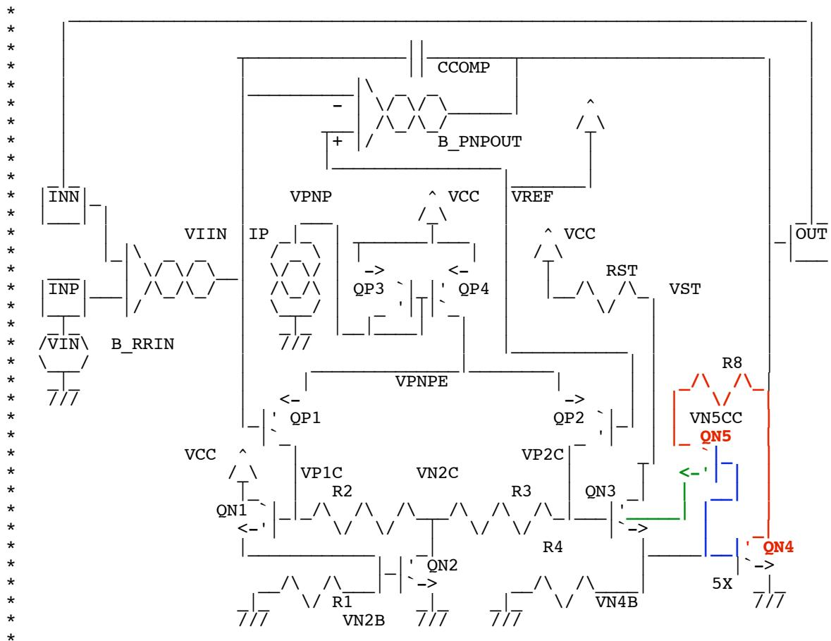
This problem can be handle by building an output transistor saturation current limit. Transistor QN5 is a reverse connected transistor which is using the collector junction as an emitter and the emitter is being used as a collector. The performance of such a transistor is not great. But since QN6 and QN4 are both npns, the "emitter base" of QN5 will turn on exactly when the collector base of QN4 turns on. Some adjustments like R8 are sometimes needed to optimize this type of current limit.
