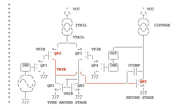
The circuit is a simplified LM324 input stage. As long as lowering the base voltage on QP2 increases the base voltage on QN3, then the amplifier is operating normally. If the base of QP2 drops enough to saturate QP2, this is no longer the case.
