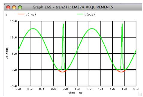
This simulation shows some of the extra features that get designed within an Op Amp that may not appear in the data sheet. If care is not taken at the input stage, swinging a few hundred millivolts below ground can cause the output voltage swing to reverse phase.
