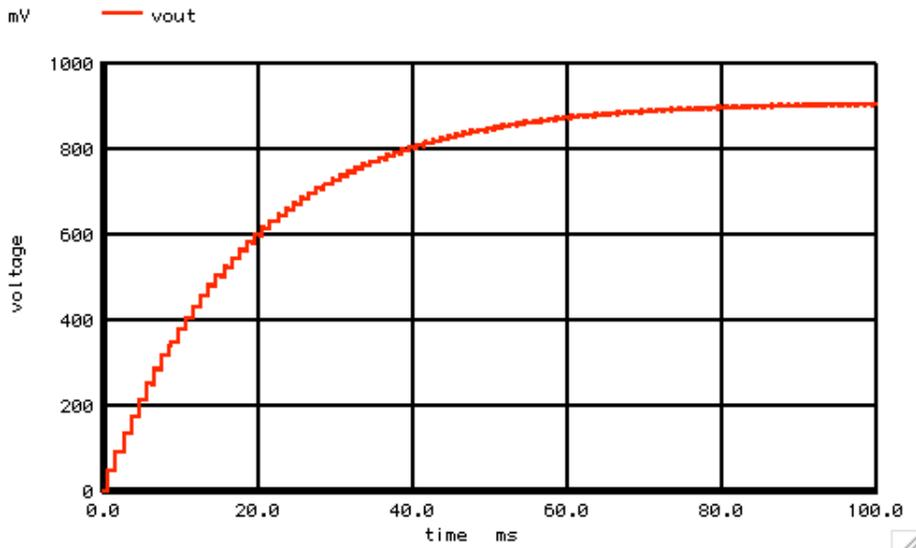
The switch capacitor should appear as a 1k Ohm resistor.
