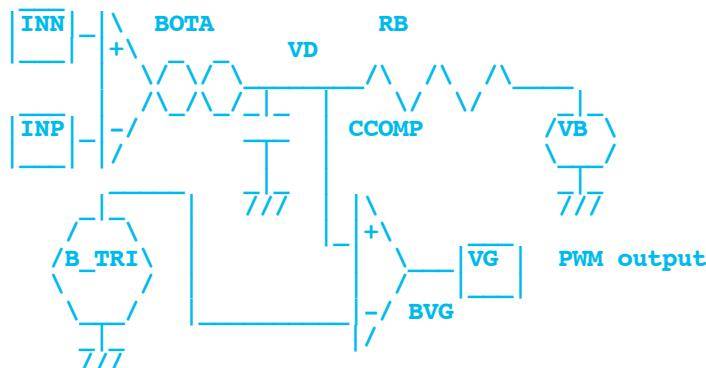
In this simulation, the Op Amp is being modeled as an input transconductance stage which has its open loop gain defined by the input transconductance and  $R_B$ , and its bandwidth is defined by the input transconductance and  $C_{Comp}$ .
