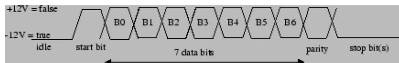
Figure 24: RS-232 Frame (1 start bit, 7 data bits, 1 parity bits,
