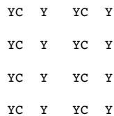
Fig.3 MPEG-2 and CCIR Rec. 601 4:2:2 organization
