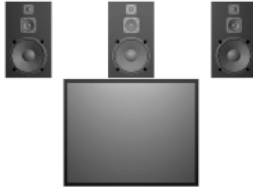
Figure 2-12 Ideal Setup - All Speakers Above Screen
