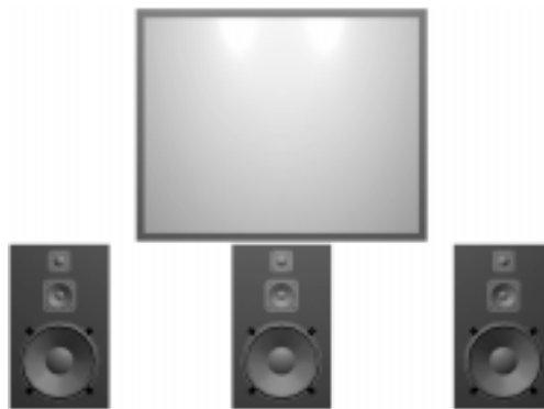
Figure 2-13 Ideal Setup - All Speakers Below Screen
