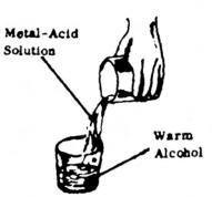
CAUTION: This reaction generates large quantities of toxic, flammable fumes. The process must be conducted outdoors or in a well ventilated area, away from sparks or open flames. Do not inhale fumes.
