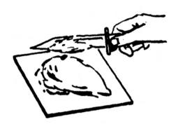
Press an aluminum plate very firmly upon the mixture on the copper plate. Remove completely any of the mixture that squeezes out between the plates. The plates must not touch.
