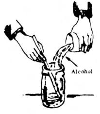
7. Filter the solution through a paper towel into a container to collect the arystals. Wash the crystals left on the paper towel three times, using 1/2 cup (120 milliliters) portions of alcohol each time.
