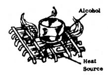
4. Pour the metal-acid solution into the warm alcohol. Reaction should start in less than 5 minutes. Dense white fumes will be given off during reaction. As time lapses, the fumes will become less dense. Allow 10 to 15 minutes to complete reaction. Fulminate will settle to bottom.
