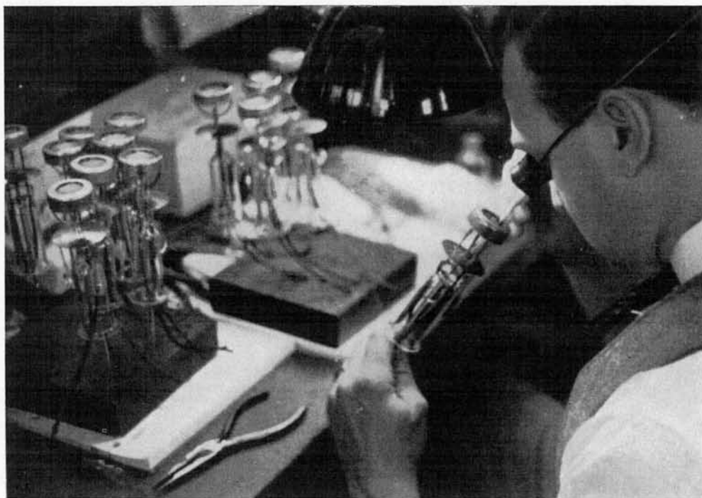
Inspecting the cathode of a mercury rectifier tube before sealing-in
